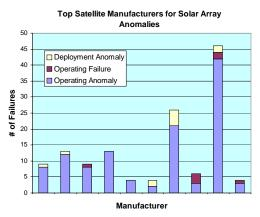
Fig. 3. Top Satellite Manufactures for anomalies
