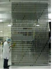
Fig. 7. A 3.75 kW Stretched lens array on a SquareRigger platform
