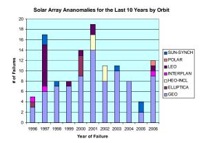
Fig. 1. Solar array anomalies by orbit
