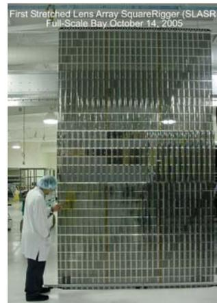
Fig. 2. Full scale SLASR panel
