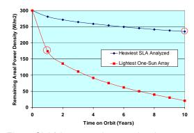
Fig. 8. SLA/planar areal power density comparison
