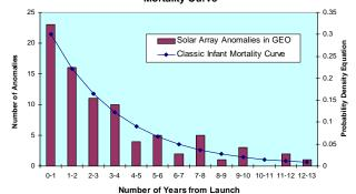
Fig. 3. Solar array anomalies compared to infant mortality curve
