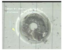
Fig. 9. Lens sample after hypervelocity shot
