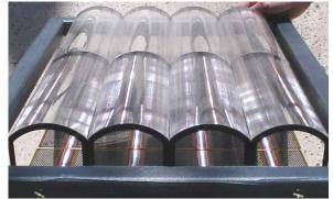
Fig. 1. Stretched lens array in sunlight
