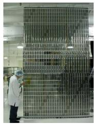
Fig. 6. 3.75 kW SLA on a SquareRigger platform
