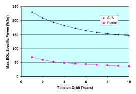
Fig. 7. EOL specific power with optimal shielding
