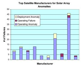
Fig. 6: Top Satellite Manufactures for anomalies
