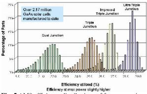
**Fig. 5** AM0 efficiency distributions of four generations of Spectrolab space solar cells.
