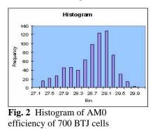
This level of efficiency represents the upper part of the efficiency histogram for the BTJ cell. The results of the
