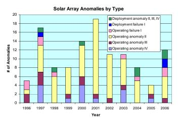
Figure 2: Solar Array Anomalies by Type
