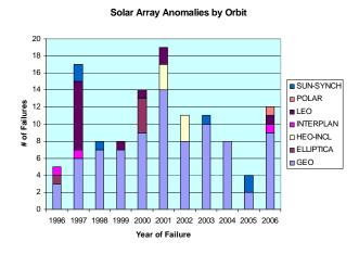
Figure 3: Satellite failures by orbit
