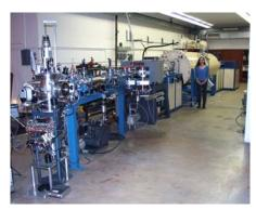
Figure 3: NEC Pellatron 2 MV Dual Source Tandem Accelerator
