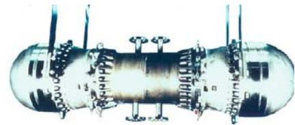
**Figure 2:** 25 kW Space Power Demonstrator Engine (ca 1992)
