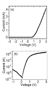
FIG. 1. (Color online) (a) Linear *I*-*V* plot of the diode with as-deposited  $ZrB_2$  Schottky contact. (b) Semilogarithmic *I*-*V* plot of the diode with as-deposited  $ZrB_2$  Schottky contact.
