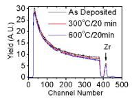
FIG. 3. (Color online) Rutherford backscattering spectroscopy of the  $\rm ZrB_2/GaN$  contact.
